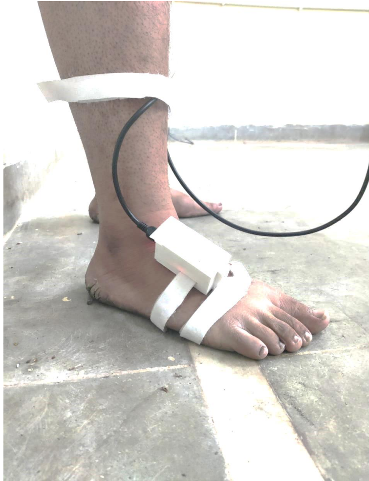
Figure 13: - Placement of the IMU sensor on metatarsal bones of the foot
