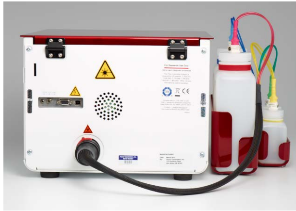
Figure 3-5. Proper Attachment of Fluidics Lines
