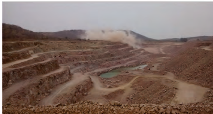
Fig 2: A view of blasting in trial blast at Dunguri mine, ACC (Case study-1)
