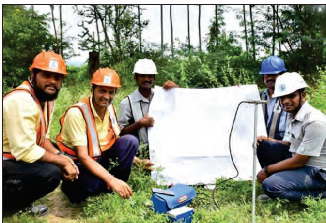
Fig 5: Monitoring of blasting operations with Minimate instrument at Jayanthipuram mine
