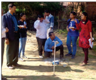
Fig 1: Instrumentation for monitoring of ground vibrations due to blasting
